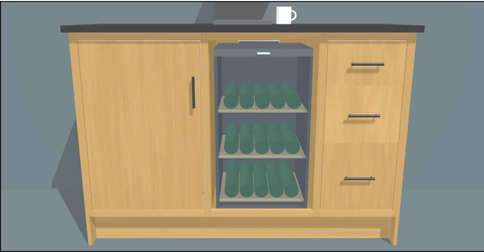
Front view, doors and drawers closed. Door and drawer fronts sit inside their openings, flush with the cabinet front.
